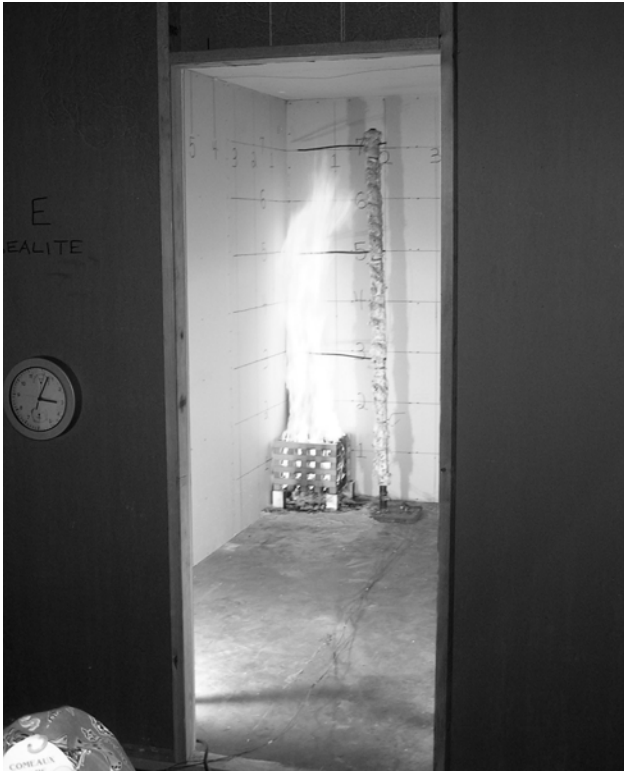
Figure 2: Photo showing UBC 26-3 testing in progress (approximately 4 minutes into a 15 minute test). Note the wood crib which provide the ignition source, the thermocouple “tree” for measuring temperature response, and the door into the 8 ft x 12 ft room.
