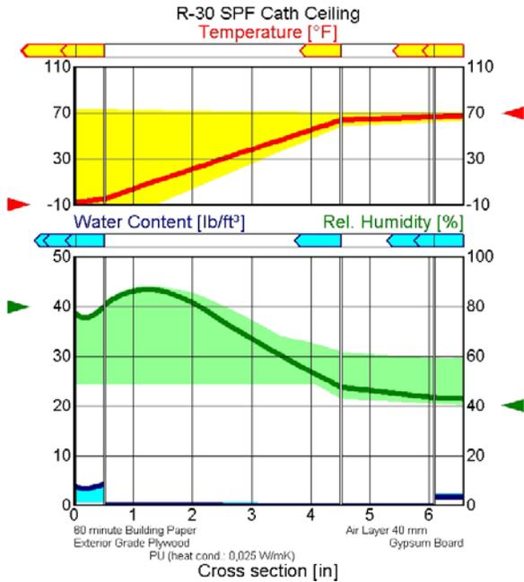
**Figure 2: Typical WUFI simulation. Top (yellow) graph represents the temperature profile, bottom (green/blue) graph is the moisture/humidity profile. The dark curves (red and dark green) are the current profiles, the shaded regions (yellow and light green) represent the range of earlier profiles. This simulation was an R-30 SPF cathedral ceiling, north facing, in Edmonton, Alberta. This simulation was run from October 1 to March 2 of the “coldest” typical year.**
