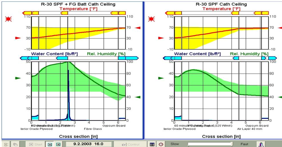
**Figure 3: “What-If” Scenario. Note high humidity levels in the left-hand chart and the blue spike indicating a high water content. The conclusion is that condensation is a potential problem in the SPF-glass fiber batt assembly whereas the all-SPF assembly is “safe.”**
